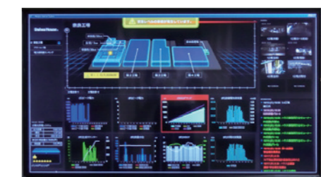
D's FEMS: Monitors not only energy data, but also data on accident prevention, labor environment and production.
