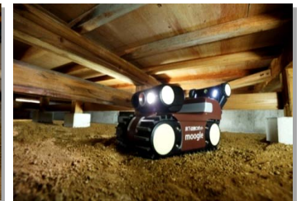
The moogles robot for inspection of crawlspace
