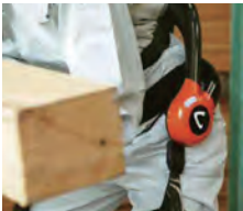
Robotic assistive harness Robot Suit HAL® for labor support (lumbar) This robotic harness alleviates the strain on a worker's lower back.
