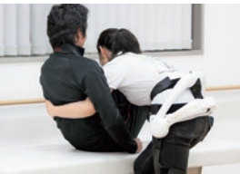
ROBOT SUIT HAL ® for care support (lumbar type)
