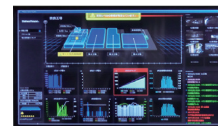
D's FEMS: Monitors not only energy data, but also data on accident prevention, labor environment and production.
