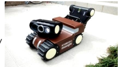
▲ Under-floor inspection robot "Moogle"
